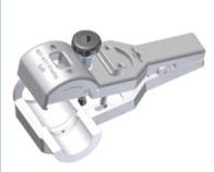
This special trimming tool improves the cable preparation prior to connector attachment. No further tools are required to prepare the cable for the connector attachment. This is due to the unique design of the trimming tool, which combines all necessary functions in one tool. It can be used for CELLFLEX® LCFS/UCF114-50 foam dielectric cables in combination with the OMNI FIT Standard connector family CO2.
