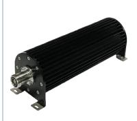
The TERP-43-product family consists of coaxial loads supporting an operational frequency band from 698MHz up to 3800MHz. The products are ideally suited for termination of unused ports in distributed antenna systems or in RADIAFLEX® radiating cables systems. The loads feature an outstanding PIM performance to avoid interferences in 3G / 4G / 5G communication systems.
