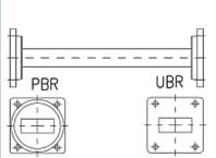
Rectangular Waveguide R 320 Straight Section, flanges PBR/UBR 320, f= 26.3-40.0 GHz, VSWR max 1.08, A=100mm (3.9in), gasket and screw kit enclosure made of copper
