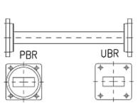
Rectangular Waveguide R 140 Straight Section, flanges PBR/UBR 140, f= 11.9-18.8 GHz, VSWR max 1.05, A=100mm (3.9in), gasket and screw kit enclosure made of copper
