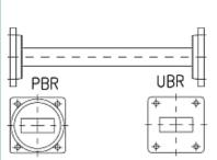
Rectangular Waveguide R 100 Straight Section, flanges PBR/UBR 100, f= 8.20-12.5 GHz, VSWR max 1.03, A=100mm (3.9in), gasket and screw kit enclosure made of brass
