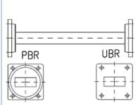
Rectangular Waveguide R 84 Straight Section, flanges PBR/UBR 84, f= 6.57-9.99 GHz, VSWR max 1.03, A=100mm (3.9in), gasket and screw kit enclosure made of brass
