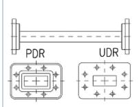
Rectangular Waveguide R 70 Straight Section, flanges PDR/UDR 70, f= 5.38-8.17 GHz, VSWR max 1.03, A=100mm (3.9in), gasket and screw kit enclosure made of brass
