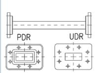
Rectangular Waveguide R 40 Straight Section, flanges PDR/UDR 40, f= 3.22-4.900 GHz, VSWR max 1.03, A=100mm (3.9in), gasket and screw kit enclosure made of brass
