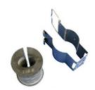
The RSB clip is designed for installation of FLEXWELL elliptical waveguide types E105 to E380 and overmoded waveguide type EO38. The clip is a universal clamp device which can be used in many mounting configurations. The clip is manufactured from stainless steel and is resistant against most environmental conditions. The set consists of a stainless steel clamp including a clamp lining made of rubber.
