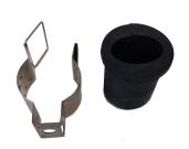
The RSB clip is designed for installation of FLEXWELL elliptical waveguide types E100 to E380. The clip is a universal clamp device which can be used in many mounting configurations. The clip is manufactured from stainless steel and is resistant against most environmental conditions. The set consists of a stainless steel clamp including a clamp lining made of rubber.
