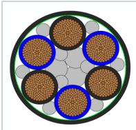
**RFS' HYBRIFLEX**  $^{\text{TM}}$  cabling solution for Remote Radio Unit (RRU) combines optical fiber and DC power in a single lightweight aluminum corrugated cable, making it the world's most innovative solution for RRU deployments. It was developed to reduce installation complexity and cost at Cellular sites.
