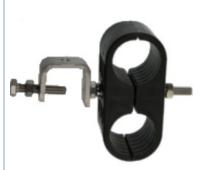
Double Multi block hanger support systems are designed for organizing bundled runs of coax cable. Each space-saving block securely holds two runs of coax, allowing a compact bundle of up to 6x runs to be supported by stacking three blocks.
