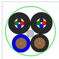
RFS' HYBRIFLEX<sup>™</sup> cabling solution for Remote Radio Unit (RRU) combines optical fiber and DC power in a single lightweight aluminum corrugated cable, making it the world's most innovative solution for RRU deployments. It was developed to reduce installation complexity and cost at Cellular sites.
