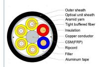
RFS HYBRIFLEX<sup>™</sup> cabling solution for Remote Radio Unit (RRU) combines optical fiber and DC power in a single lightweight aluminum corrugated cable, making it the world's most innovative solution for RRU deployments. It was developed to reduce installation complexity and cost at Cellular sites.
