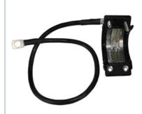
This Grounding Kit has been developed by RFS for the CELLFLEX® cable series. The Grounding Kit body facilitates a proper attachment to the coaxial cable, ensuring that the performance of the coaxial cable is not being compromised. The tin plated copper mesh provides a secure, low resistance contact to the cable outer conductor. The installation only takes a few minutes. No additional sealing with mastic and electrical tape required.
