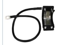
This Grounding Kit has been developed by RFS for the CELLFLEX $^{\otimes}$  cable series. The Grounding Kit body facilitates a proper attachment to the coaxial cable, ensuring that the performance of the coaxial cable is not being compromised. The tin plated copper mesh provides a secure, low resistance contact to the cable outer conductor. The installation only takes a few minutes. No additional sealing with mastic and electrical tape required.
