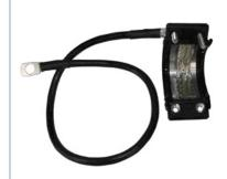
This Grounding Kit has been developed by RFS for the CELLFLEX® cable series. The Grounding Kit body facilitates a proper attachment to the coaxial cable, ensuring that the performance of the coaxial cable is not being compromised. The tin plated copper mesh provides a secure, low resistance contact to the cable outer conductor. The installation only takes a few minutes. No additional sealing with mastic and electrical tape required.
