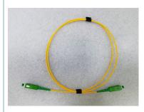
A simplex fiber optic patch cord incorporating bend insensitive single mode fiber, preterminated with SC/APC connectors on both ends. The tight buffered fibre and non metallic strain member is protected by an LSZH jacket, suitable for indoor applications
