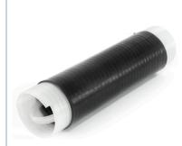
COLD-022-W cold shrink tubes are open-ended tubular EPDM rubber sleeves, pre-expanded on a removable core for easy installation. After the core is removed, the tube shrinks to its original diameter guaranteeing a perfect sealing on connectors.
