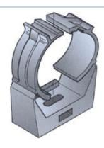
Clic Clamp, 1/2" RADIAFLEX polyamide black, halogen free Fire class UL94HB UL746C rated material suitable for outdoor applications
