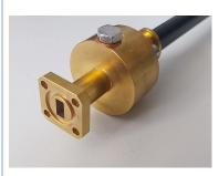
Standard connector for FLEXWELL® elliptical waveguide E300 with PBR320 flange, gasket with shrinking sleeve sealed frequency range: 27.5 - 33.4 GHz
