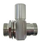
This 7-16 DIN style hybrid quarter wave surge arrestor with gas capsule for high-power and low IM application is foreseen for bulkhead mounting or in-line arragement with grounding wire connection (not included) via M8 thread.
